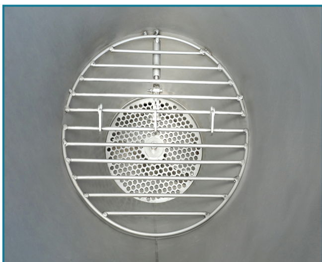
If the hopper's grid is not locked, the RotoSift will not run. Safety with every function.
